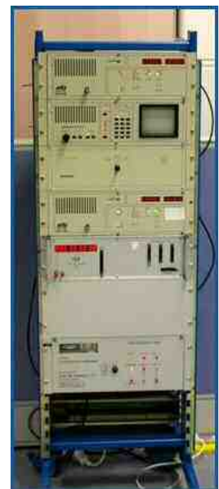
Computerised equipment incorporating voice synthesis that finally replaced the 1954 Speaking Clocks
