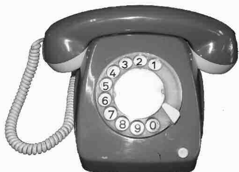
Siemens Table Set as used in Argentina (similar in appearance to the Australian 800 series)
