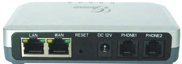
The Grandstream HT-502 is a two (telephone) port ATA that supports pulse dialling.
